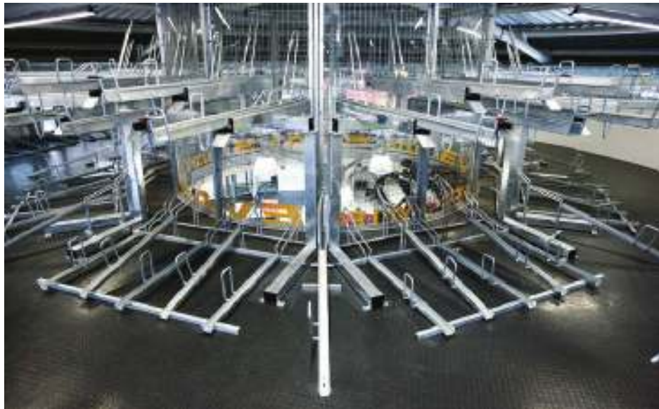
Leeds CyclePoint (above and right) is an automated parking system
